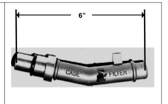
6. Install oil filter into case:
