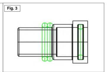
5. Lubricate the O-rings with ATF and push the extension tube onto the transmission end of your stock oil pick-up tube. Push the extension tube onto the pick-up tube until it stops against the shoulder on the pick-up tube.
