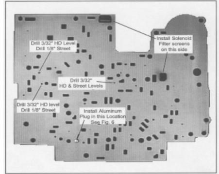
Figure 5. Separator Plate
