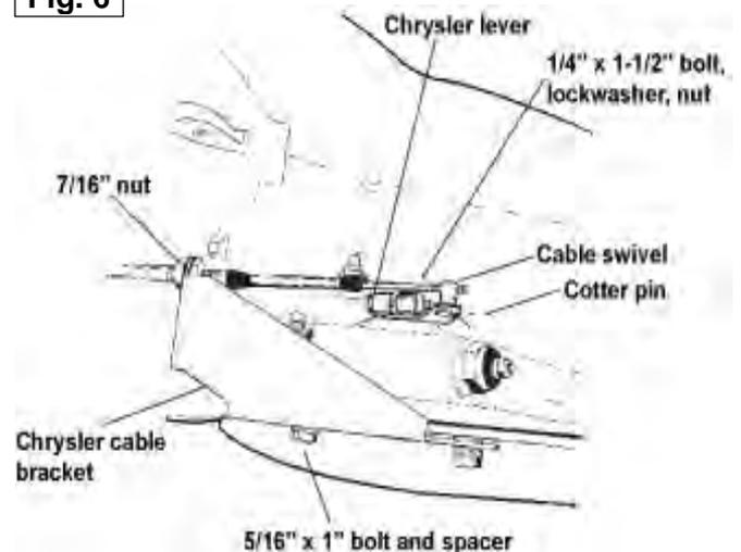
20. Remove the two transmission oil pan bolts directly below the shift lever. Install the cable bracket in position (See Fig. 6) with two spacers between the pan and the bracket. (If your transmission is equipped with a cast aluminum oil pan these spacers can be omitted.) Install the two 5/16-18 x 1.00" pan bolts supplied and tighten to 12-13ft.lbs. Do not overtighten as this can damage the pan gasket.
