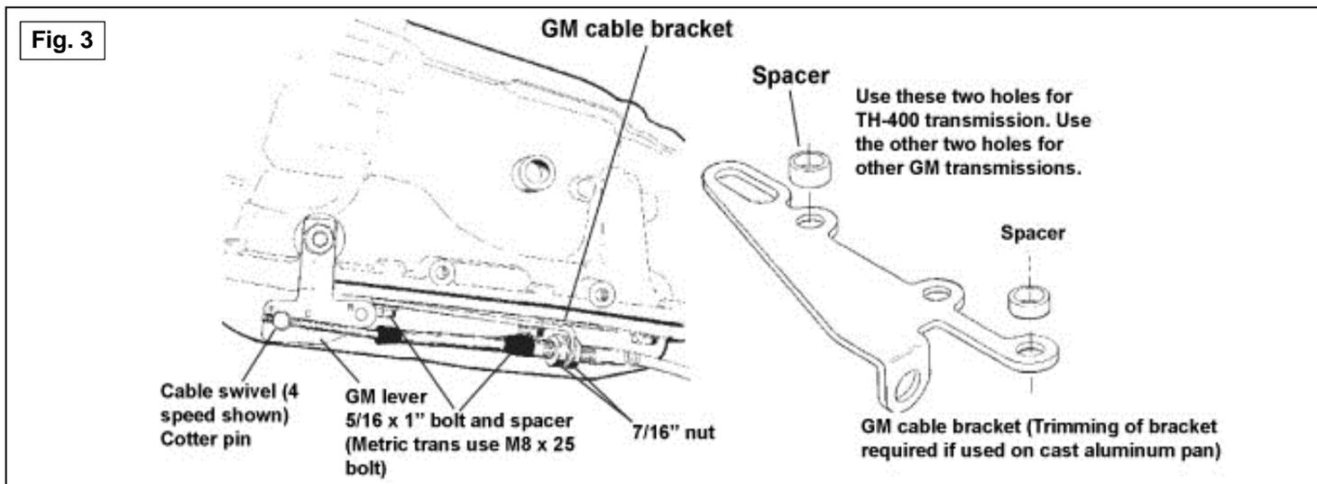
11. Move the transmission selector lever by hand to full rear position (Low). Operate the shifter lever to the Low gear position (ratcheted all the way back). Adjust the large nuts on the cable so that the swivel will slide into the center hole on the selector lever. Tighten the large nuts completely. Be sure that the swivel will slide freely in and out of the hole in the selector lever.
