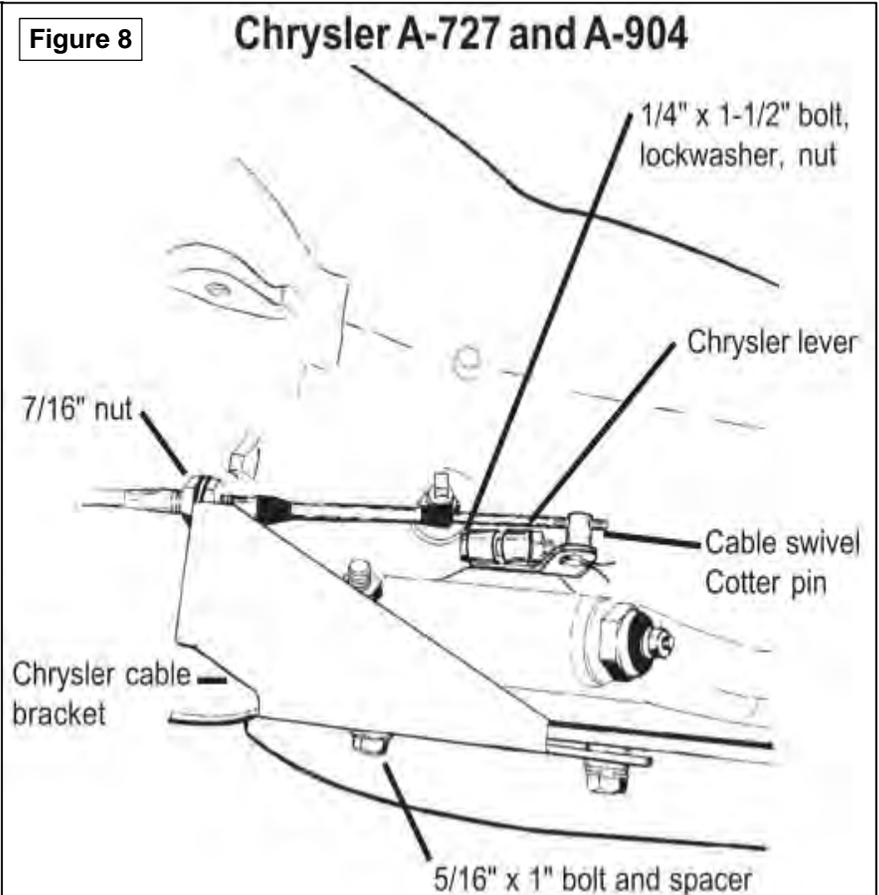
22. Remove the two transmission oil pan bolts directly below the shift lever. Install the cable bracket in position with the two spacers between the pan and the bracket (See Figure 8). (If your transmission is equipped with a cast aluminum oil pan these spacers can be omitted.) Install the two 5/16-18 x 1.00" pan bolts supplied and tighten to 12-13 lb.ft. Do not overtighten as this can damage the pan gasket.
