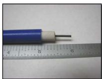
After you have measured and cut the wire(s) to the correct length, strip back  $\frac{1}{2}$ " of white insulation surrounding the center core, *without damaging the core*! Next, cut and strip 3/8" of colored outer jacket without cutting into the white inner insulation. Next, carefully fold over the center core. Insert the wire into the terminal with the core next to the bottom of the terminal and form the terminal tabs around the wire to hold it in place for crimping.
