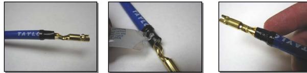
Put some of the silicone grease on the terminal and heat shrink tubing. Spread it around the terminal to aid the installation into the distributor boot.
