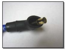
For the early style socket type terminal, put a slight bend in the terminal to aid in the boot installation. Insert the terminal/wire into the boot. Carefully bend the terminal up into a 90 degree configuration to fit the boot correctly. (You <u>do not</u> have to bend the terminal when using the late model HEI style boot/terminals).
