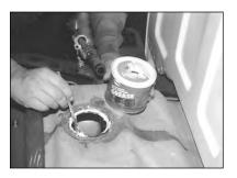
Install the complete assembly back in the fuel tank. Make sure you don't bend anything while reinstalling. Lock assembly back in place by rotating lock ring clockwise until it hits its stops. Now tighten fuel connections and hose
