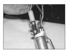
on the pump. Some shortening of the rubber hose may be necessary for proper alignment of the pump with the pump hanger.
