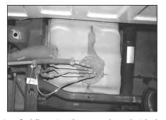
assembly. Disconnect two fuel lines, two hoses, and an electrical connection with a ground wire. There is a center fuel pump sending unit assembly lock ring holding the assembly into the tank.
