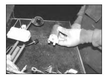
**NOTE:** There is a kit supplied with the new fuel pump. Install the 3" length of fuel hose onto the 3/8" steel tubing where the old fuel pump junction hose was previously. Use the 3/8" hose clamp to secure hose to steel tubing. The fuel line will be a very tight fit over the 3/8" tubing. It may be necessary to lube the tubing with some spray lubricant to ease hose installation. You must use the supplied 3" length of hose. DO NOT use the stock rubber fuel hose.
